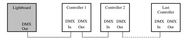
In this configuration controller 1 is set in mode 10; all the others are set in mode 1.
