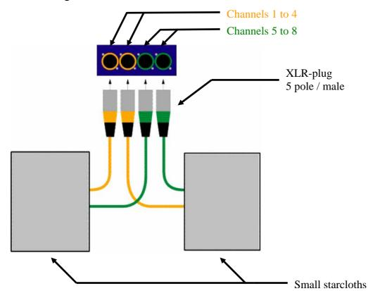
Note: The connectors with the same colour code are switched in parallel (internally)
